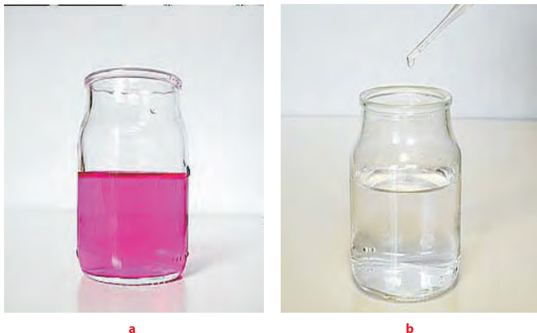
Figure 2.2 The colour changes of phenolphthalein in basic (a) and acidic (b) solutions.
